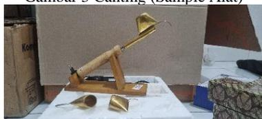
Gambar 4 Canting Listrik (Sample Alat)
